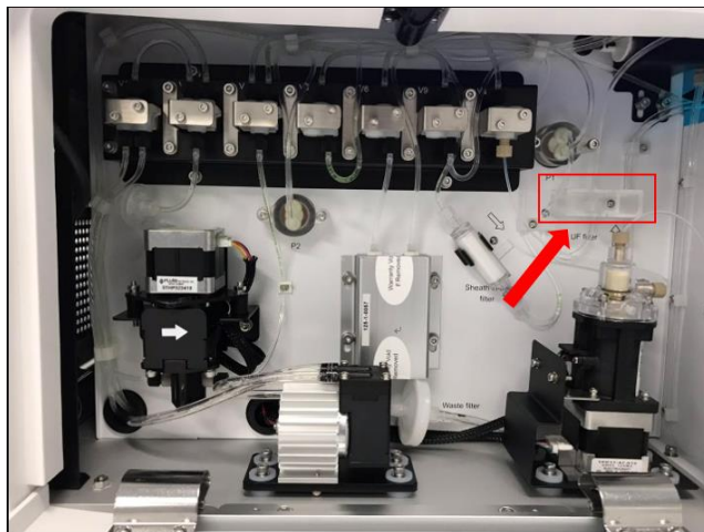
Figure 102. Location of the 0.05 µm Sheath Fluid Ultrafiltration (UF) Filter rack
